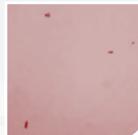
Quality steel. The inclusions are globular with some sharp edges. This steel does not break (it is tough) although the inclusions affect the characteristics of the steel.
